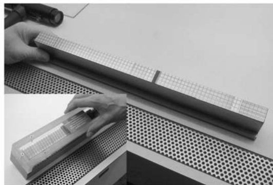
Fig. 5 Typical silicon single-crystal substrate for FEL application: plane mirror, T-mount, 500 mm long. The insert shows the same mirror after deposition. A strip of the 45 nm thick carbon coating is visible in the middle of the surface.
